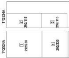
Cutting steel reinforcement mesh
